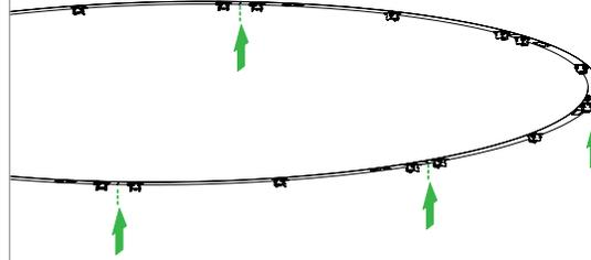
INSTALL ALL TOP PLATES AND BRACKETS TO CEILING AND ENSURE THEY ARE FLAT BEFORE INSTALLING THE FIXTURE.
