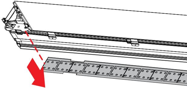
REMOVE CARTRIDGES FROM FIXTURE
