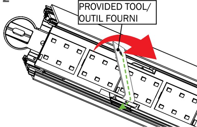
USE PROVIDED TOOL OVER LOCK SPRING TO REMOVE ELEMENTS
