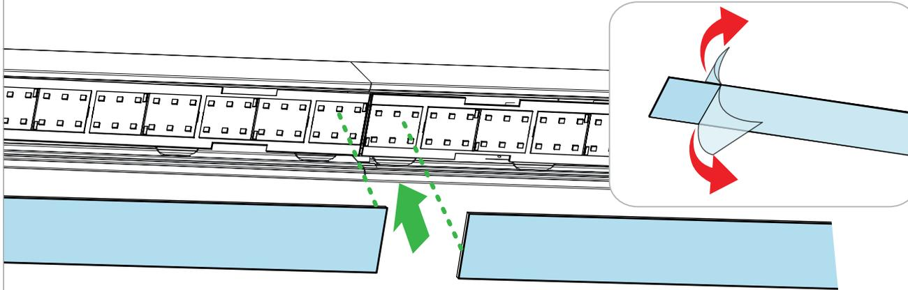
REMOVE PROTECTIVE FILM FROM BOTH SIDES OF LENS AND INSTALL IT BY SNAPPING IN WITH **MATTE SIDE FACING OUT.**
