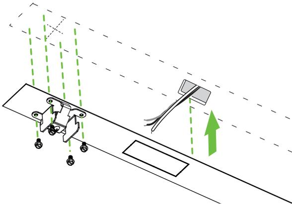
INSTALL TOP PLATE AND BRACKETS TO CEILING. MAKE NECESSARY ELECTRICAL CONNECTIONS TO FIXTURE.
