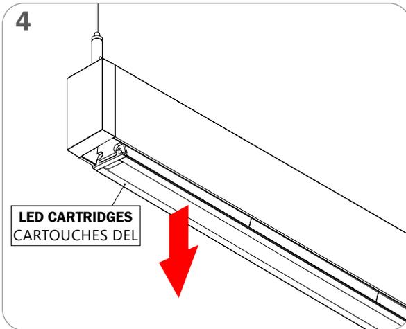
**CONTINUOUS ROW:** FOLLOW STEPS 1 TO 3 TO INSTALL NEXT FIXTURE IN CEILING AND REMOVE CARTRIDGE
