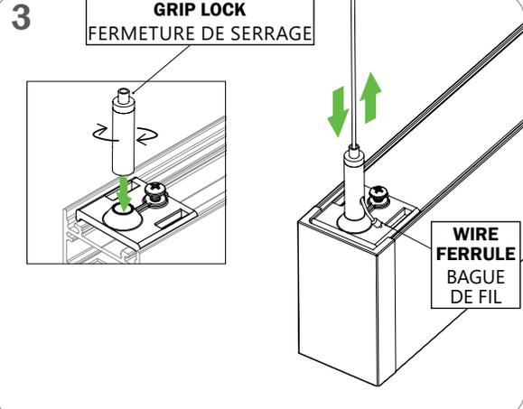
**LEVEL THE FIXTURE STRAIGHT BY PRESSING ON THE GRIP LOCK WHILE MOVING THE FIXTURE UP AND DOWN**
